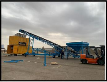
Belt conveyor system can transport materials in bulk and bagged, such as stone, sand, coal, concrete, cement, gravel, fertilizer, mineral ore, limestone, coke, sawdust, wood chip, bulk material, grain, corn flakes, carbon black, etc.
